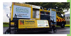
We invested in an ultra eco-friendly thermal road repair system. This sustainable technology makes repairs using an infra-red heating process which reheats the existing road surface, bringing it back to a workable state where it can be recycled and used again Additional material is added, mixed in and compacted to reform the road back to a high standard.
